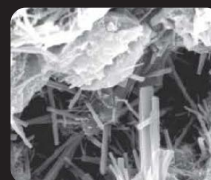
Crystal growth in concrete after application of crystals forming waterproofers.
