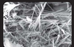
Fully developed crystal growth at 28 days within the capillary tracts of concrete to block flow of water.
