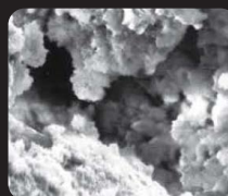
No crystal forming waterproofers present. Untreated concrete. Open pore structure.
